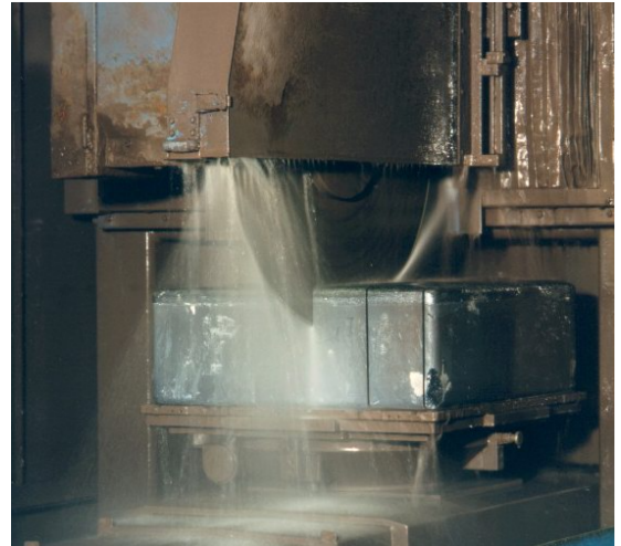
(b) The ingots of silicon must then be sliced into smaller blocks, which are later cut up into wafers through wire saws.
