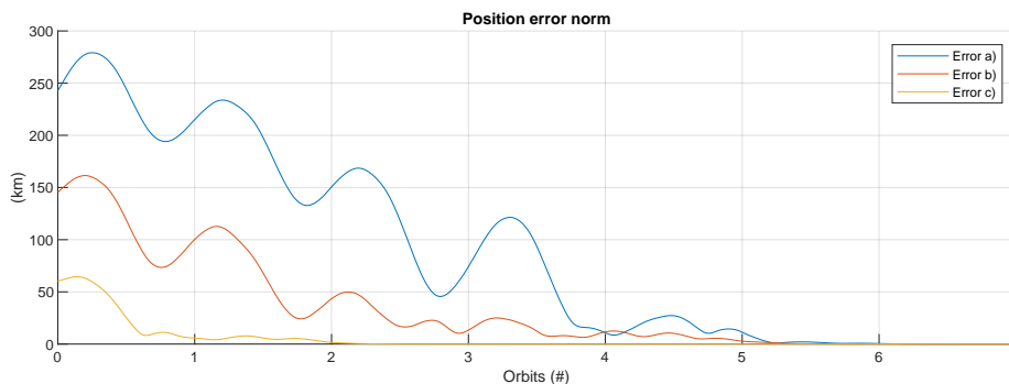
Figure 6.17: Magnitude of the position error for initial errors defined in Table 6.2.
