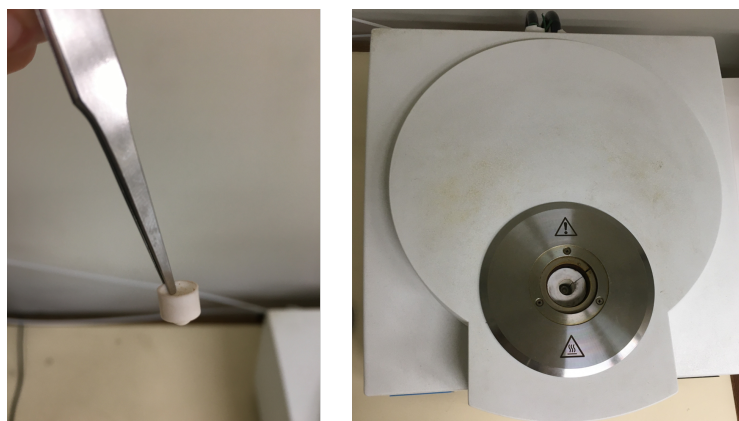
Figure 3.5: Crucible used and furnace where it was placed.
