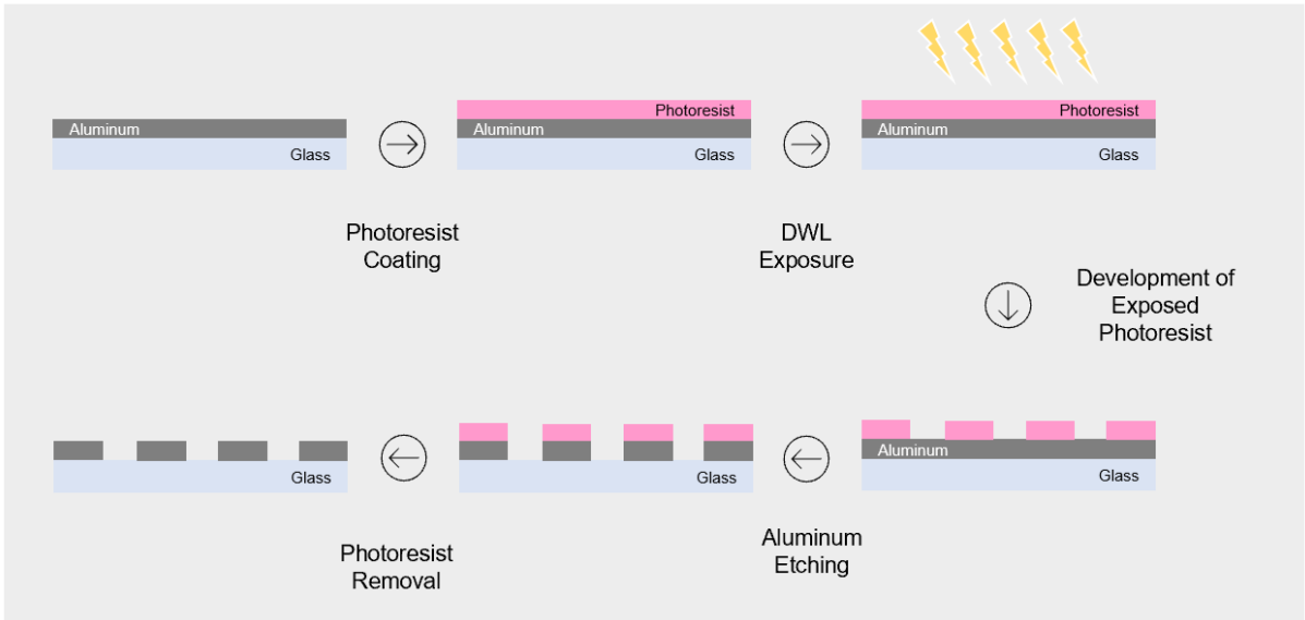
Figure 9 - Schematics of hard mask fabrication (side view). Elements not to scale.
