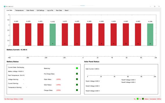
Figure 5.7: GUI while battery is being balanced.
