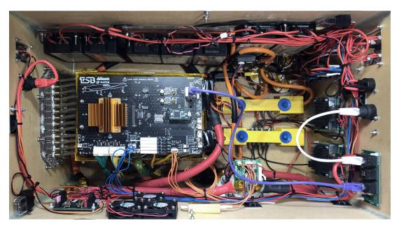
Figure 6.1: BMSSPV V2 integrated in SR-03's battery box.
