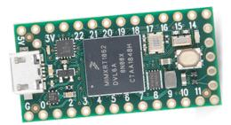
Figure 4.1: Example of a Teensy board, in this case the Teensy 4.0.
