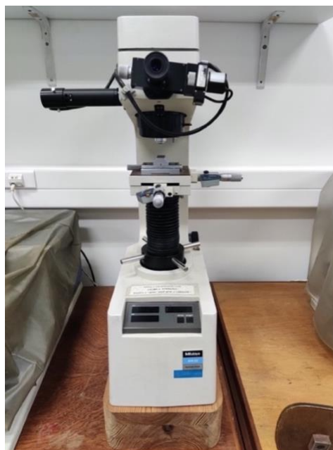
Figure 3.10- Equipment used to perform the hardness tests (Mitutoyo AVK-C2 Hardness Tester).
