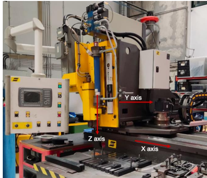
Figure 3.2- ESAB LEGIOTM 3UL- FSW equipment used in the development of the experimental work.
