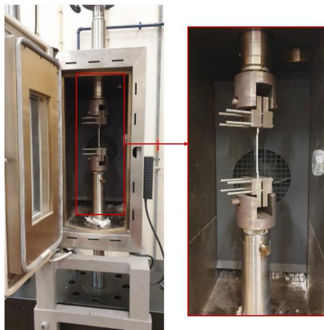
Figure 4.18- Setup used to perform the fatigue tests at 150^\circ\text{C} .
