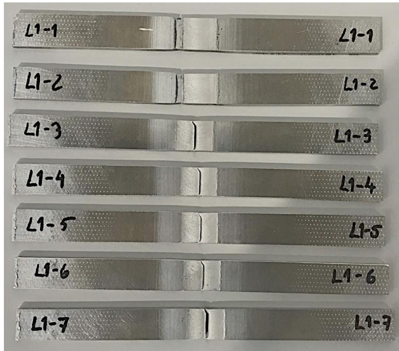
Figure 3.8- Tensile specimens obtained from the L1 weld, used in the preliminary uniaxial quasi-static tensile tests.
