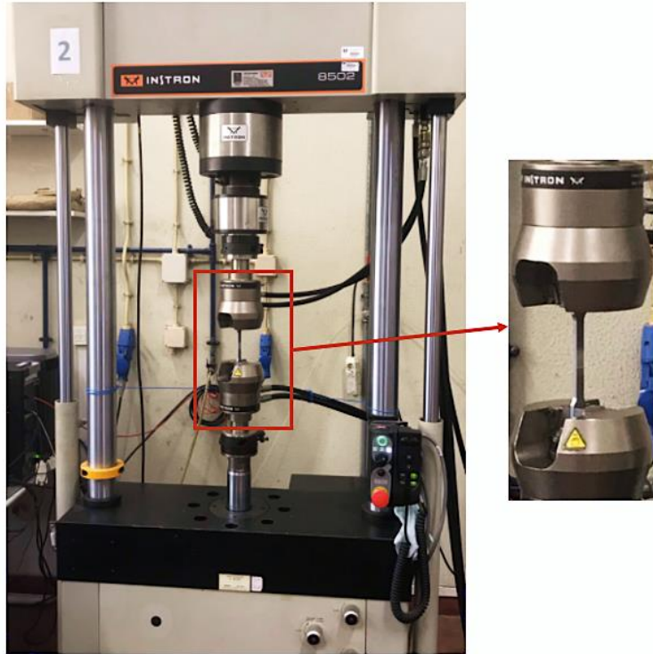
Figure 3.13- Fatigue equipment used in the execution of the fatigue tests (Instron 8502).
