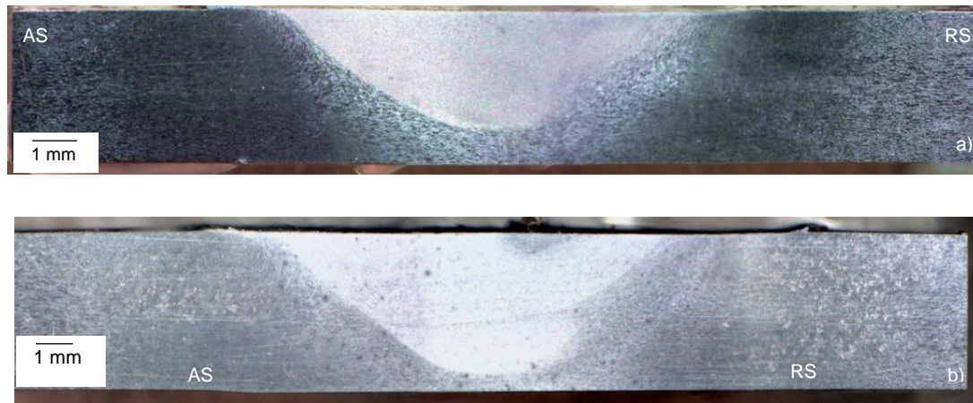
Figure 4.1- Macrographs obtained for the a) L1 weld sample and b) D13 weld sample.
