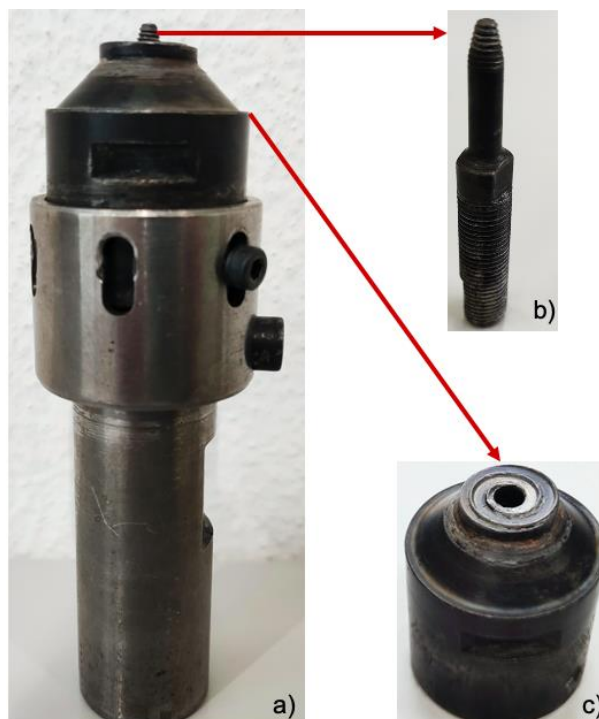
Figure 3.4- Tool (iSTIRtool_v3) used in the production of the welds: a) 3-part assembly; b) Conic Pin; c) Shoulder.
