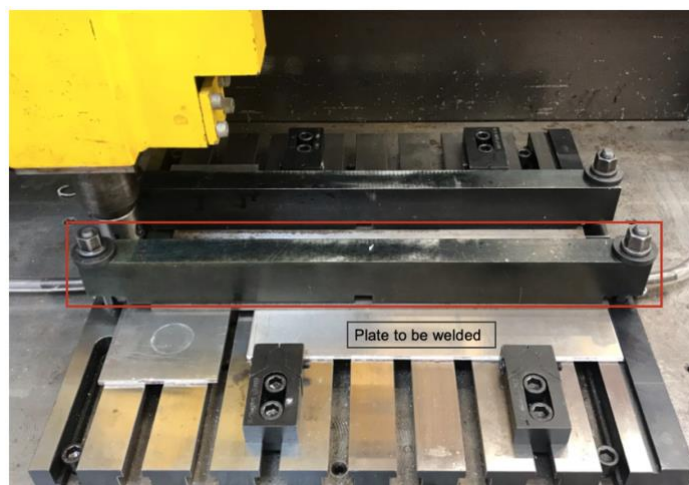
Figure 3.3- Clamping system used in the production of the welds (one of the steel bars highlighted in red).
