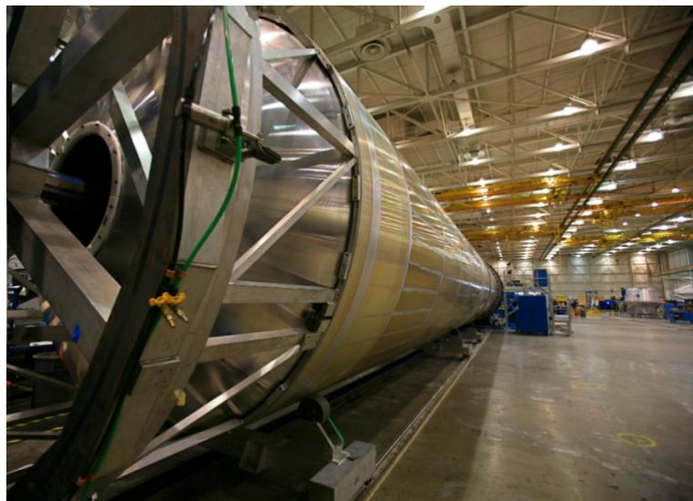
Figure 2.14- Friction stir welds on the propellant tank walls of the Space X Falcon 9 [35].
