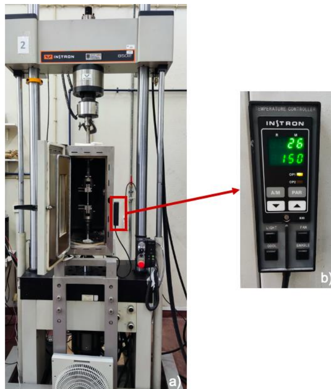
Figure 3.14- a) Setup used to perform the fatigue tests at 150 °C; b) Temperature Controller.
