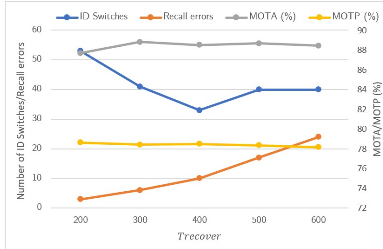
Figure 5.4: Evaluation metrics on the Re-ID Multi-Tracking Dataset when varying the value of T_{recover} . MOTA and MOTP are given in percentages and ID switches and recall errors are the total number of these occurrences on the complete dataset. The values of the other parameters are: S_{max} = 0.05m , (T_{lower}, T_{upper}) = (300, 700)
