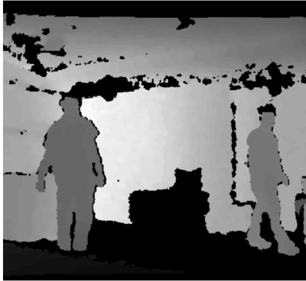
Figure 3.5: Depth image showing two people. In this image, a brighter colour represents points that are further away from the camera. Totally black represents a NaN point where the depth could not be obtained. We can see here that a person is surrounded by background points that have bigger depth.
