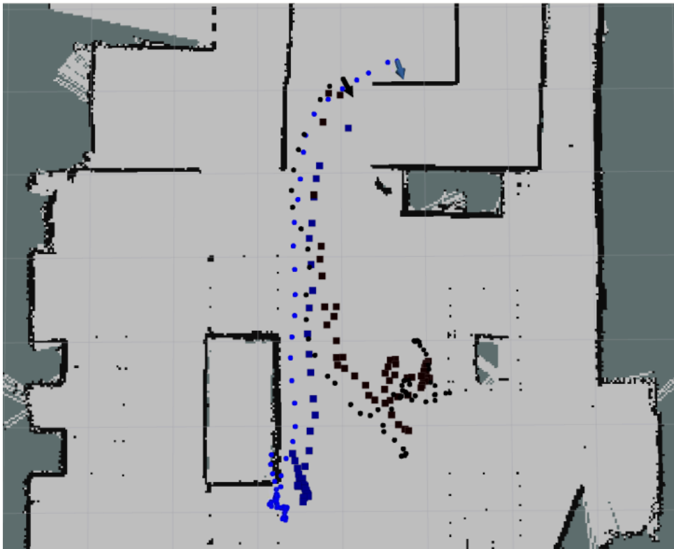
Figure 7.1: Still sequence trajectories In this figure we can see the trajectories of two targets, represented by the colors blue and black. The two tracks generated by the system show a good estimation of the target's position and there are no ID switches.
