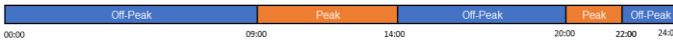
Fig. 6. Saturday periods defined by ERSE for weekly cycle tariffs during summer time
