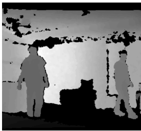
Fig. 3: Depth image showing two people. In this image, a brighter colour represents points that are further away from the camera. Totally black represents a NaN point where the depth could not be obtained. We can see here that a person is surrounded by background points that have bigger depth.
