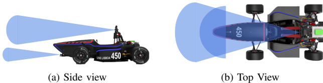
Fig. 1: Location and field-of-view of LiDAR and Camera.
