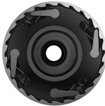
Figure 2.12 – Schematic of a pawl-style freehub with four spring loaded pawls.
