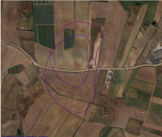
Figure 5.27: Flight path measured during the first flight.
