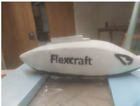
Figure 4.19: Fuselage with applied filler and paint.
