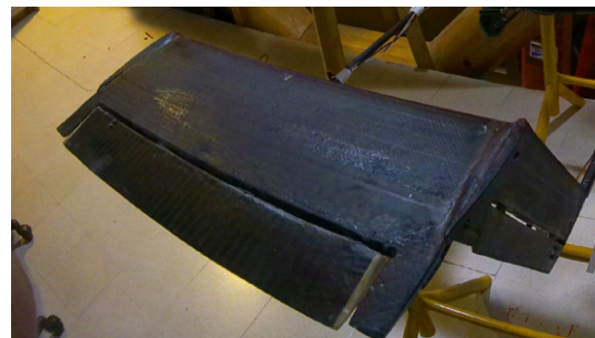
Figure 4.12: XPS with carbon reinforcement elevator and rudder mounted in F-02.
