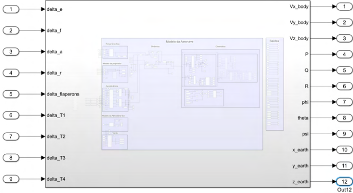
Figure 2.22: Implementation of the full nonlinear aircraft model in SIMULINK.
