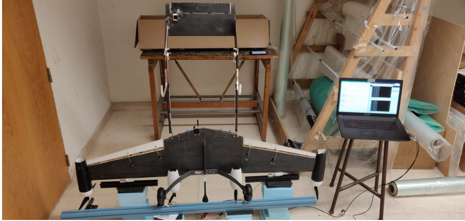
Figure 5.4: Experimental measurement of the z coordinate of the center of mass
