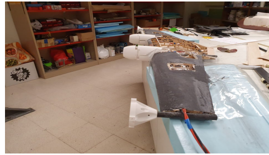
Figure 4.14: Engine mount in lateral motor and complete nacelle in central motors.
