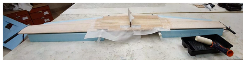
Figure 4.9: Main wing with the balsa wood skin and the lamination with glass fiber.
