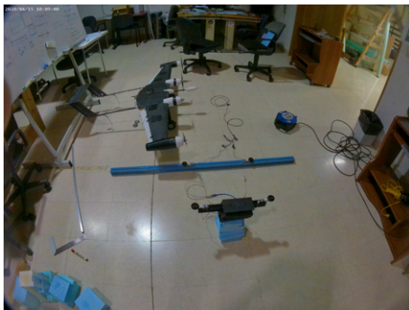
Figure 5.1: Experimental measurement of the x and y coordinate of the center of mass.
