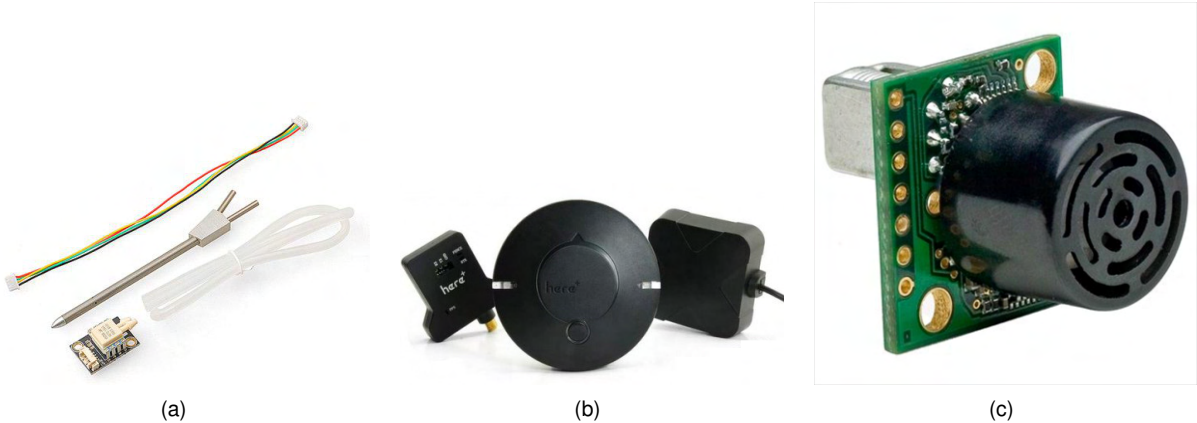
Figure 4.26: External sensors, right to left: (a) Airspeed sensor and pitot (b) GPS receiver and ground station (c) Sonar sensor.
