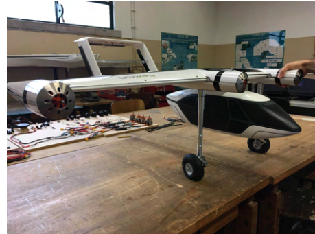
Figure 4.5: Front Landing Gear mounted in F-01 UAV.
