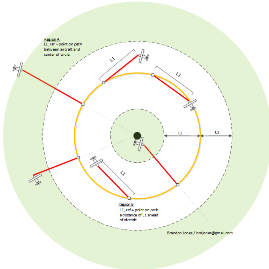
Figure 3.6: Illustration of the L1 algorithm along a circular trajectory.
