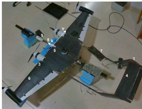
Figure 5.22: Measurement points illustrated in the F-01 UAV
