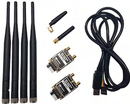
Figure 4.24: Long range RC (radio controller)/Telemetry transmitter and receiver (RFD868x bundle modem)
