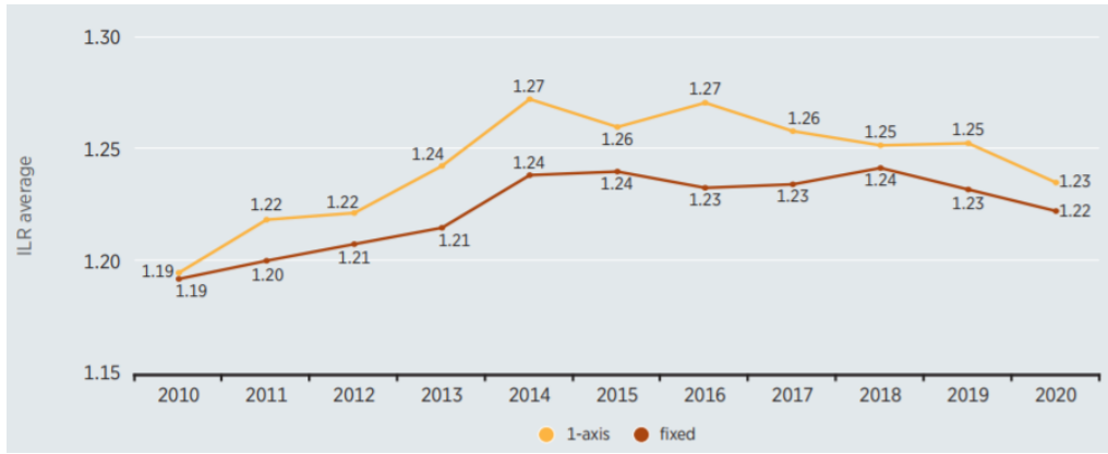
Figure 25 - Global average inverter load ratio trend, 2010-2020 [2]
