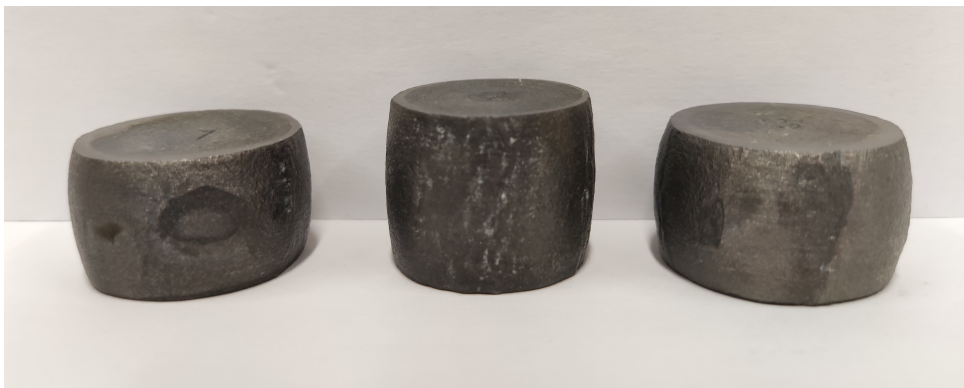
Figure 4.6: Compression specimens after being tested.
