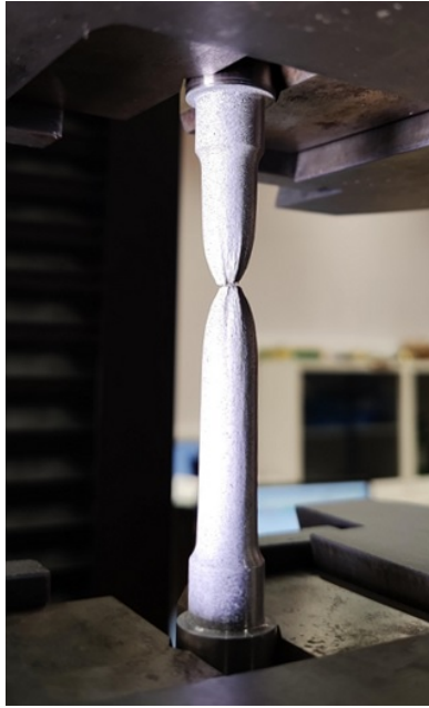
Figure 4.1: Tensile specimen after being tested.
