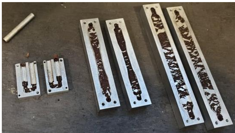
Figure 42 - Condition of the dies after an attempt to cure the non-dried polymer.
