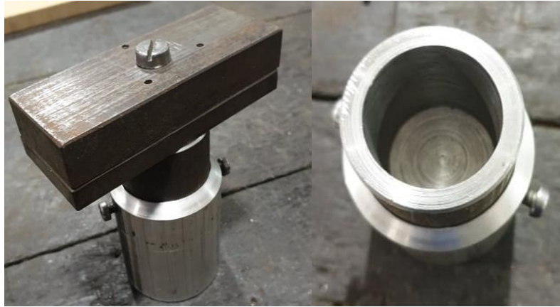
Figure 26 - The cast used to determine whether the polymers were thermosetting or thermoplastic.
