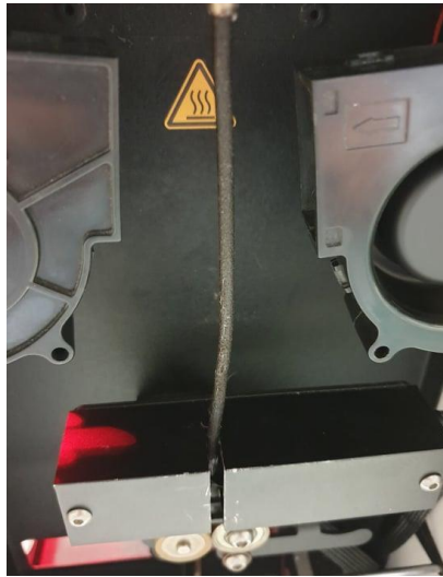
Figure 37 - Optical sensor responsible for measuring the diameter of the filament being extruded.
