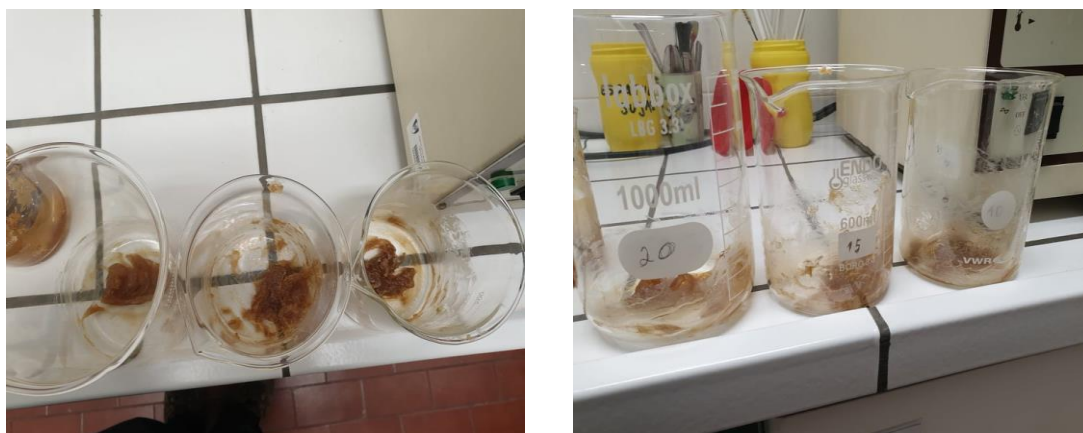
Figure 15 - Comparison of glycerine/ corn starch polymer containing 20g, 15g, 10g glycerine to 10g corn starch, respectively.
