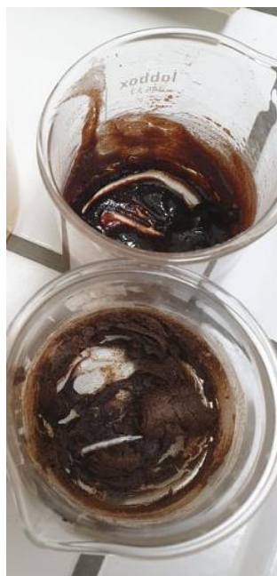
Figure 40 - Polymer in the ratio 2:1 on top and 1:1 on the bottom, with sawdust, after curing in the oven.
