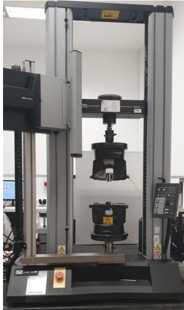
Figure 27 - The Instron 5566 Universal Testing Machine, used to perform all of the mechanical tests.
