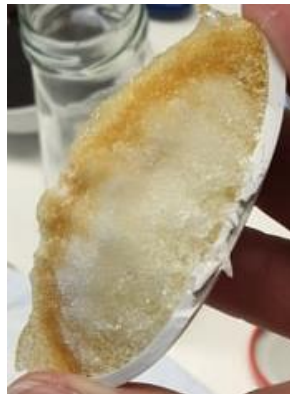
Figure 38 - Polyglycerol citrate 2:1 after curing in the microwave for 10 minutes at 700W, whereby it can be seen that the interior of the preparation was only partially polymerised.
