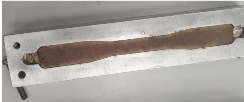
Figure 43 - Specimen for tensile test after curing in the oven for 12 hours at 140/150°C. Composite with 16.67% of sawdust by mass was used.
