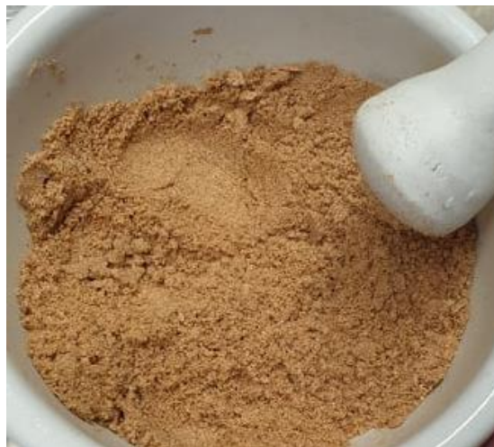
Figure 24 - Corn-starch/ glycerine/ sawdust composite prepared in the mortar, before being deposited in the dies.
