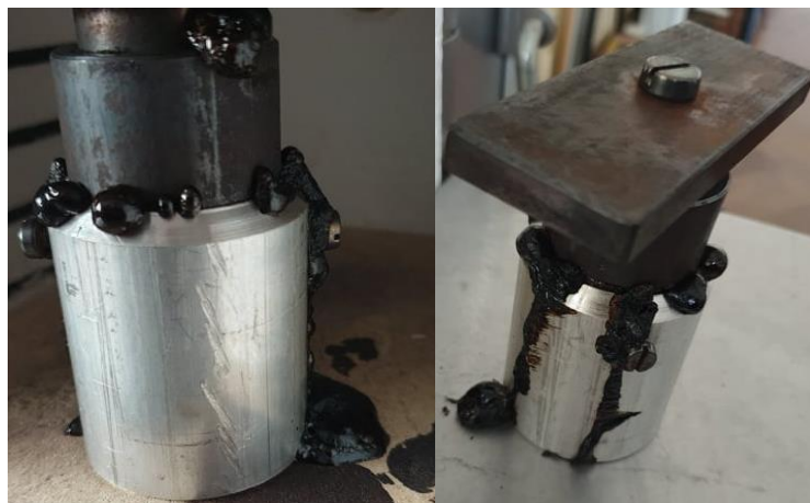
Figure 47 - Sawdust/ Corn Starch/ Glycerine composite after the test in which it was found to be a thermoplastic.
