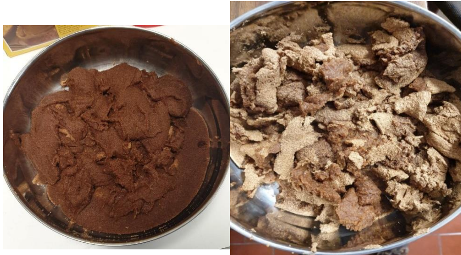
Figure 22 - Pre-polymer with wood, before drying in the oven. In the first image, the viscous solution is fresh off the hotplate and in the next one after 1 hour in ambient air.
