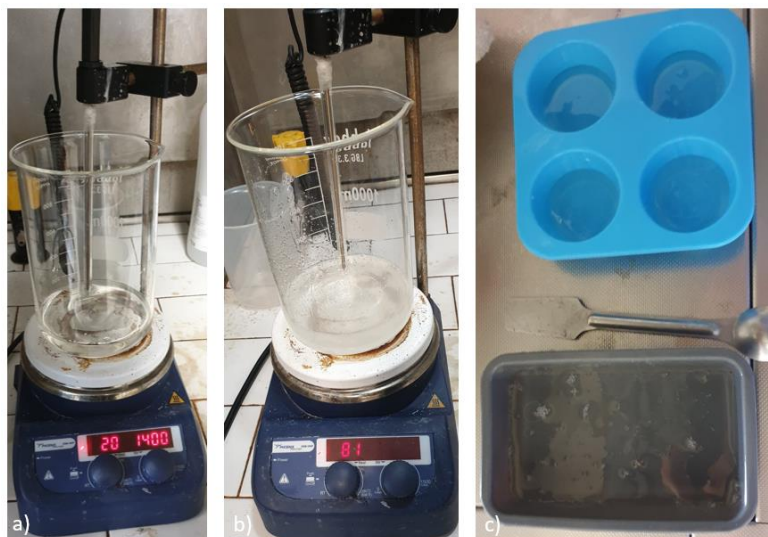
Figure 16 - Polymer preparation: a) heating glycerine; b) with citric acid added to the reaction; c) pre-polymer ready to go to be cured.
