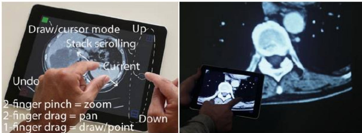
Figure 12. Touch display with interface to the left. Combination of PC screen projection and mobile device on the right. Adapted from [9].
