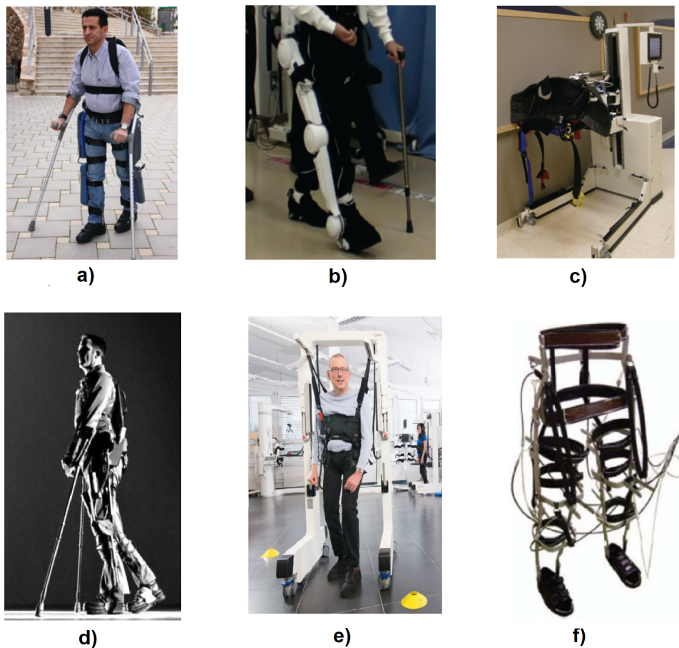
Figure 2.4: Some of the currently developed overground gait trainers. a) Rewalk from [1] b)HAL from [1] c)KineAssist from [1] d)EKSO from [9] e)ANDAGO [8] f)RGTW from
