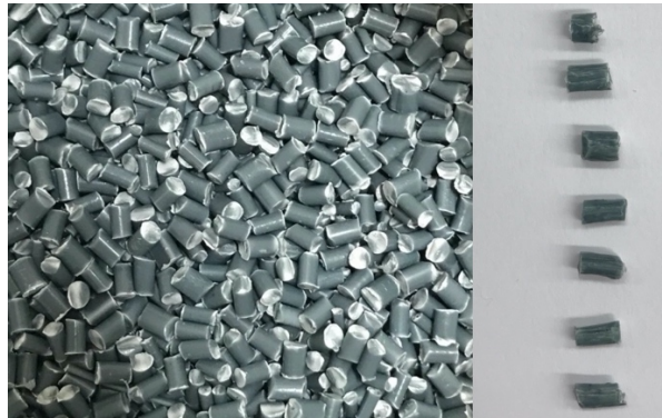
Figure 30: Comparison of pellets obtained from rPP(cmp) with separation process (left) and without separation process (right).
