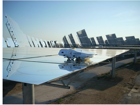
Figure 1: Heliostat cleaning with HECTOR at the Gemasolar solar power plant [5].
