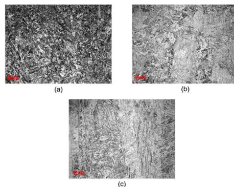
Figure 10 Microstructure in (a) - bottom portion of the sample, (b) - middle portion of the sample, (c)- top of the sample
