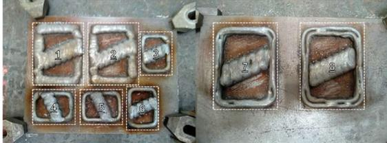
Figure 12 Experiments performed for the part deposition with PowerMill Additive
