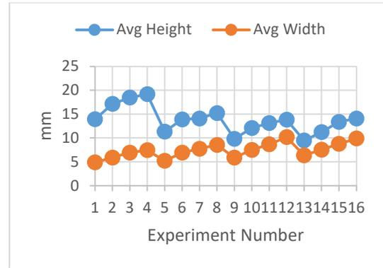
Figure 5 Average width and height of depositions
