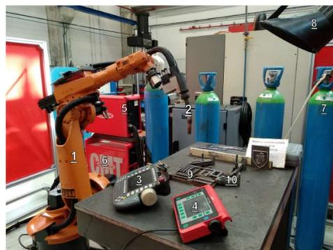
Figure 1 Deposition work setup
