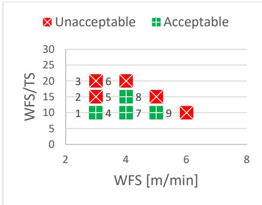
Figure 7 Visual evaluation of second set of depositions
