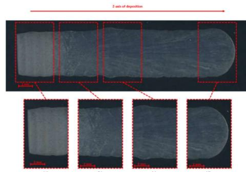
Figure 9 Macrostructure of a section of a deposition
