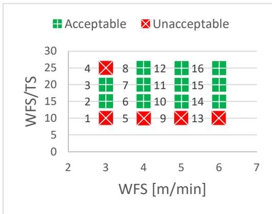
Figure 4 Visual evaluation of first set of depositions
