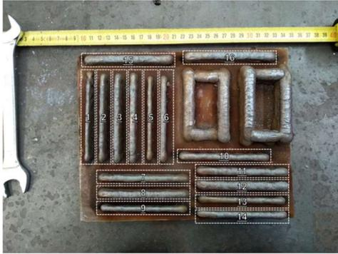
Figure 3 First set of depositions
