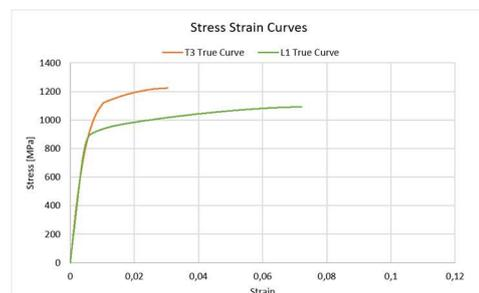
Figure 11 True stress-strain curves of samples T3 and L1
