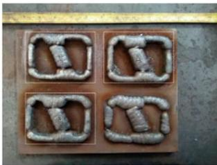
Figure 13 Experiments performed for part deposition with WAAMPlanner
