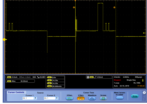
Figure 7: Oscilloscope image for a Spreading Factor of 12 with the wake up time
