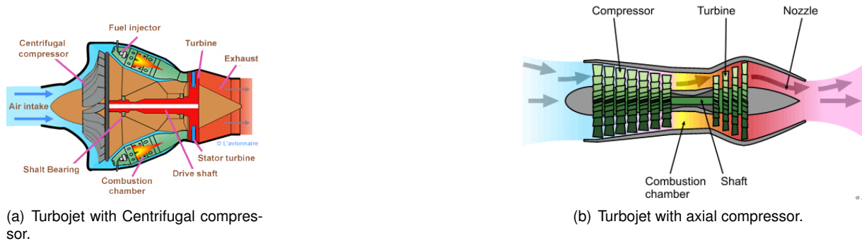
Figure 2.6: Typical compressors configurations in Gas Turbines.
