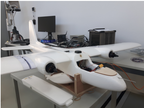
Fig. 4. The MyTwinDream UAV with its propeller blades removed.
