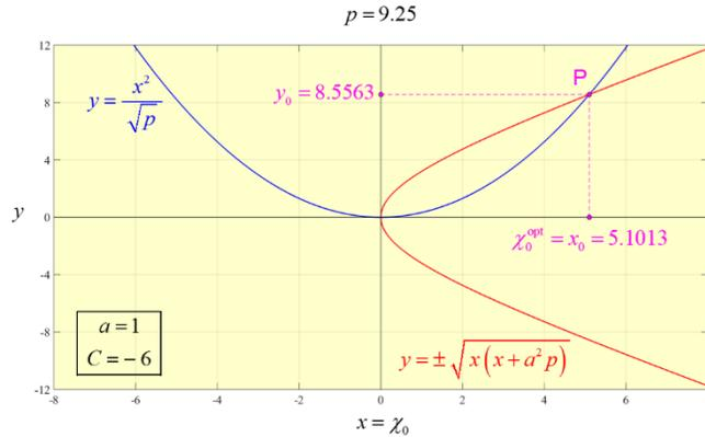
**Figure 2:** Graphical solution of the cubic equation presented in Equation (79) for  $C = -6$  and  $a = 1$ .
