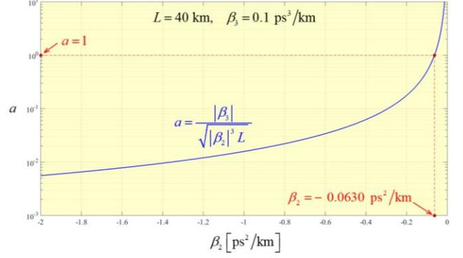
**Figure 1:** Variation of the adimensional coefficient  $a$  with the group-velocity dispersion parameter  $\beta_2$  for an optical fiber with  $L = 40 \text{ km}$  and a higher-order dispersion parameter  $\beta_3 = 0.1 \text{ ps}^3/\text{km}$ .
