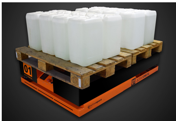
Figura 1.1: Automated Guided Vehicle (AGV) ActiveOne XL , fonte: ActiveSpace Automation. [3]
