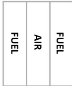
Figure 2: Schematic top view of the multi-slit rectangular burner.
