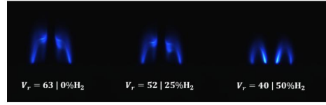
Figure 10: Evolution of flame Type II ( \phi = 0.3 ) with H_2 addition on fuel.
