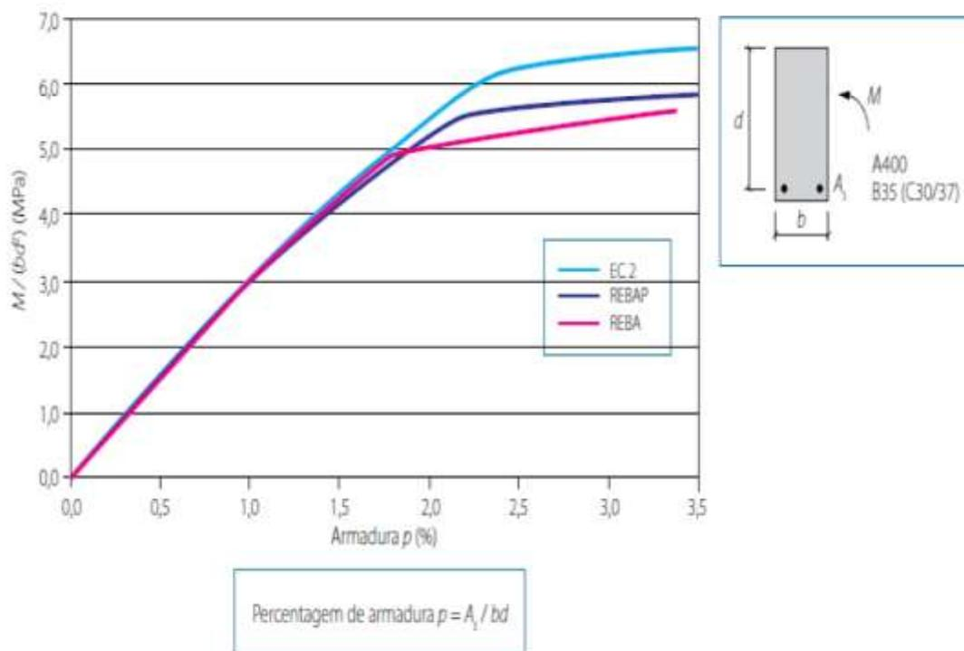
Figure 2 - Comparative analysis of the simple flexural strength of REBA (1967), REBAP (1983) and EC2 (2010) [2].
