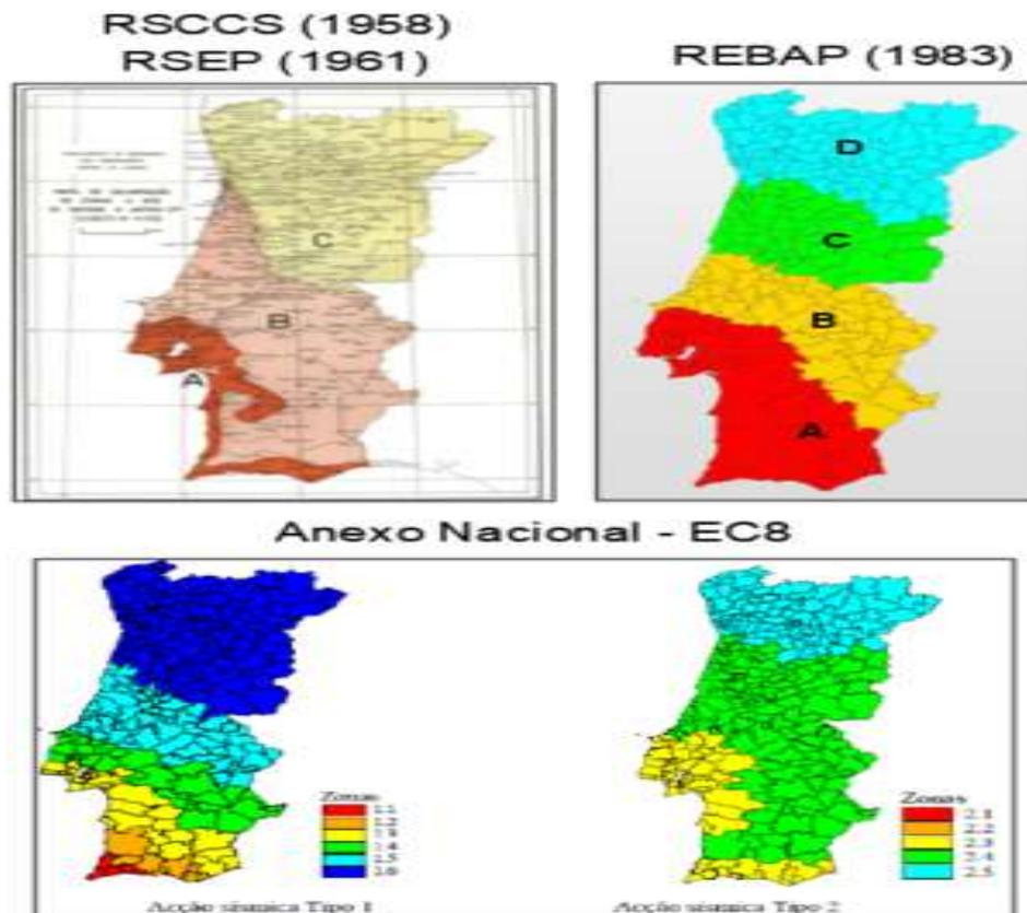
Figure 1 – Evolution of seismic action zoning in Portugal (adapted) from [2].
