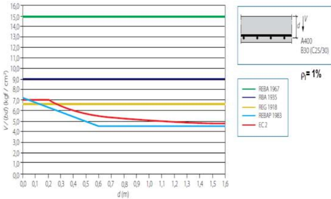
Figure 3 - Comparative analysis of resistance to transverse stress of elements without transverse reinforcement [2].
