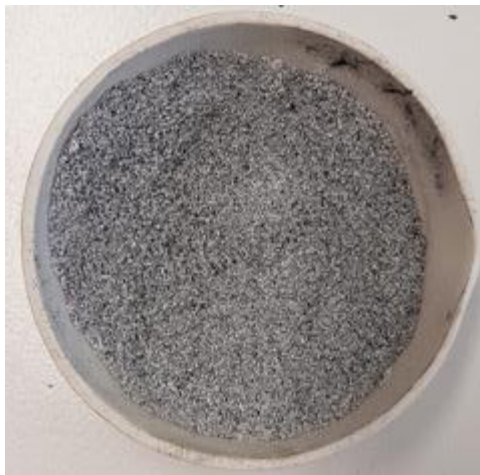
Figure 11 The sample of tyres mixed with a catalyst before pyrolysis.
