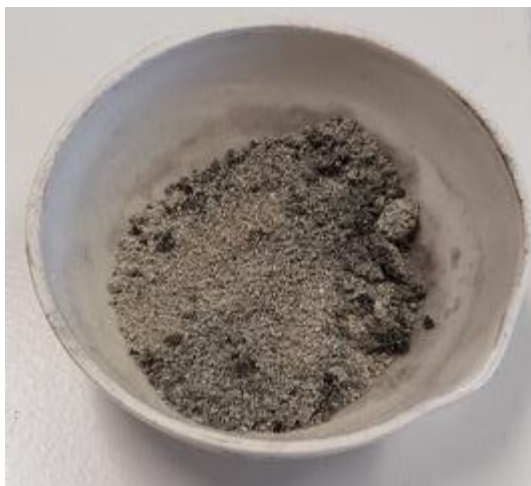
Figure 12 Bio-char after pyrolysis of rubber tyres mixed with a catalyst.
