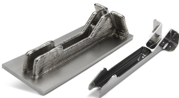
Figure 2.5: Part produced by Norsk Titanium, before and after final machining process. Source: The Fabricator magazine.
