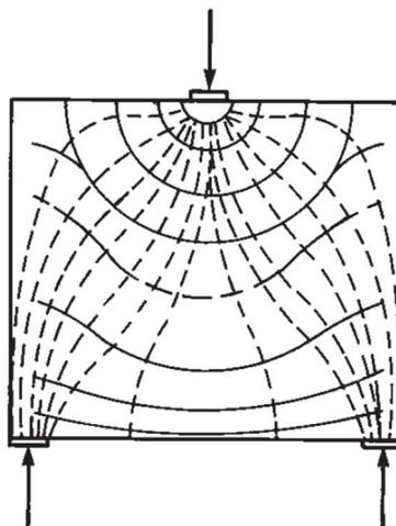
*Figure 1 Stress fields inside a deep beam subject to a point load*
