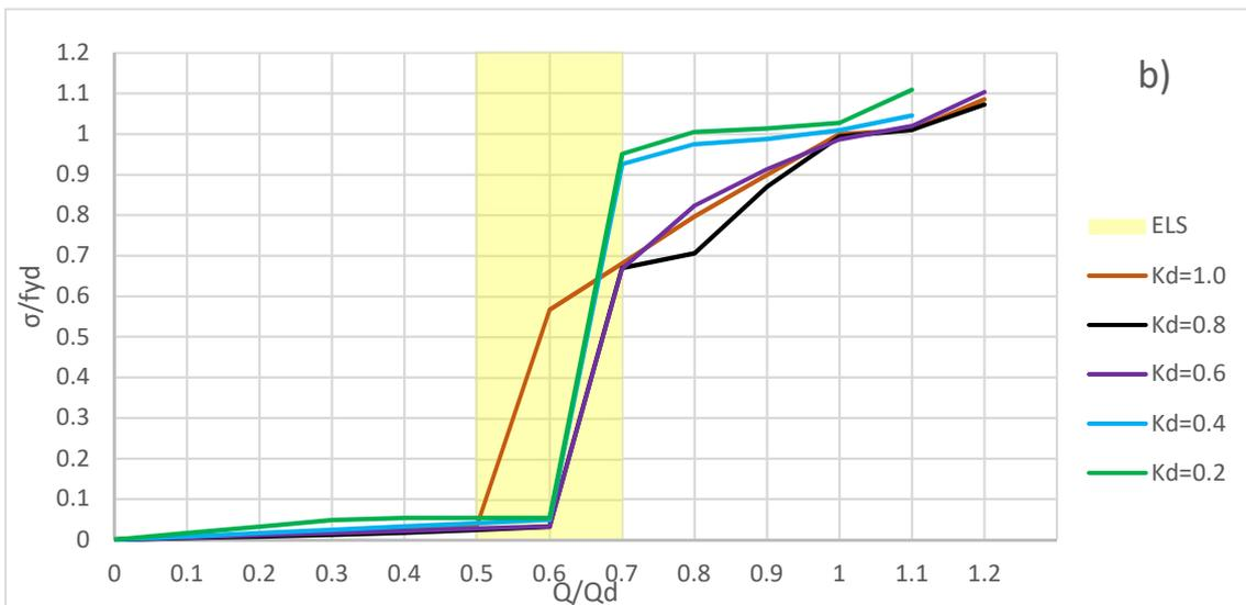
Figure 7 Stress levels on the vertical steel reinforcement (for each load step and case study)
