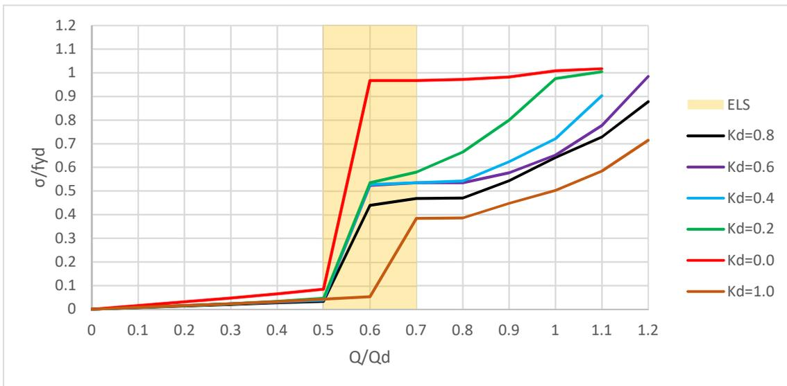
Figure 9 Stress levels on the horizontal steel reinforcement (for each load step and case study)
