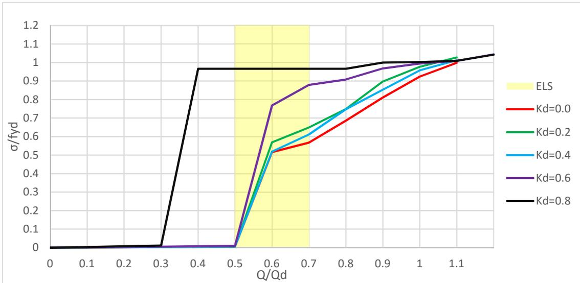
Figure 8 Stress levels on the diagonal steel reinforcement (for each load step and case study)
