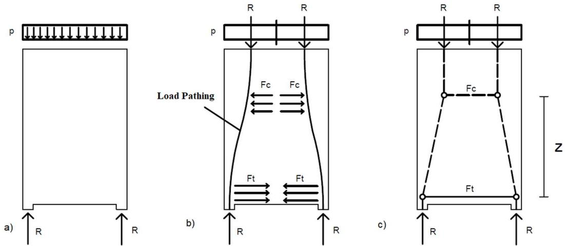
Figure 2 Application of the Load Path Method for the design of a Strut and Tie Model
