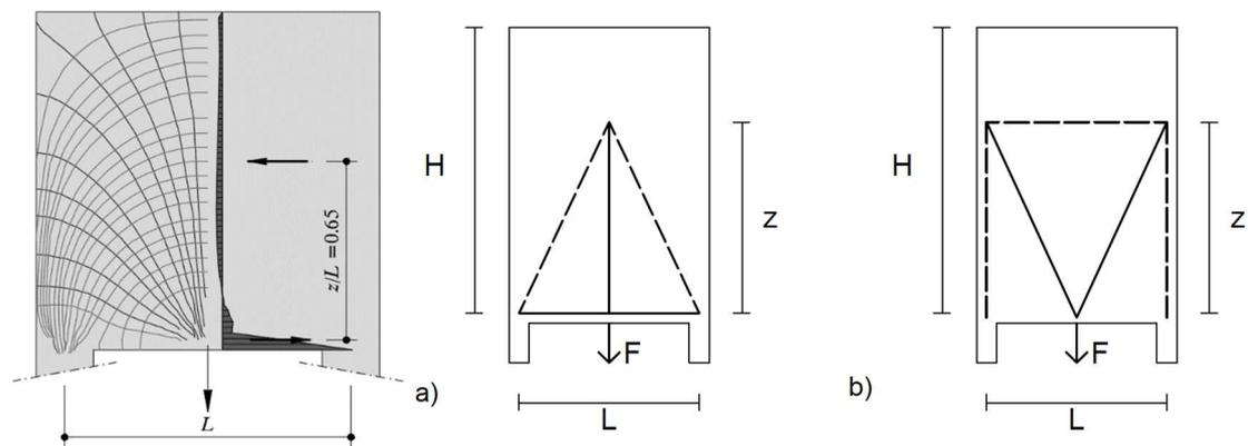
Figure 3 STM for a deep beam subject to an indirect point load and the respective elastic trajectories
