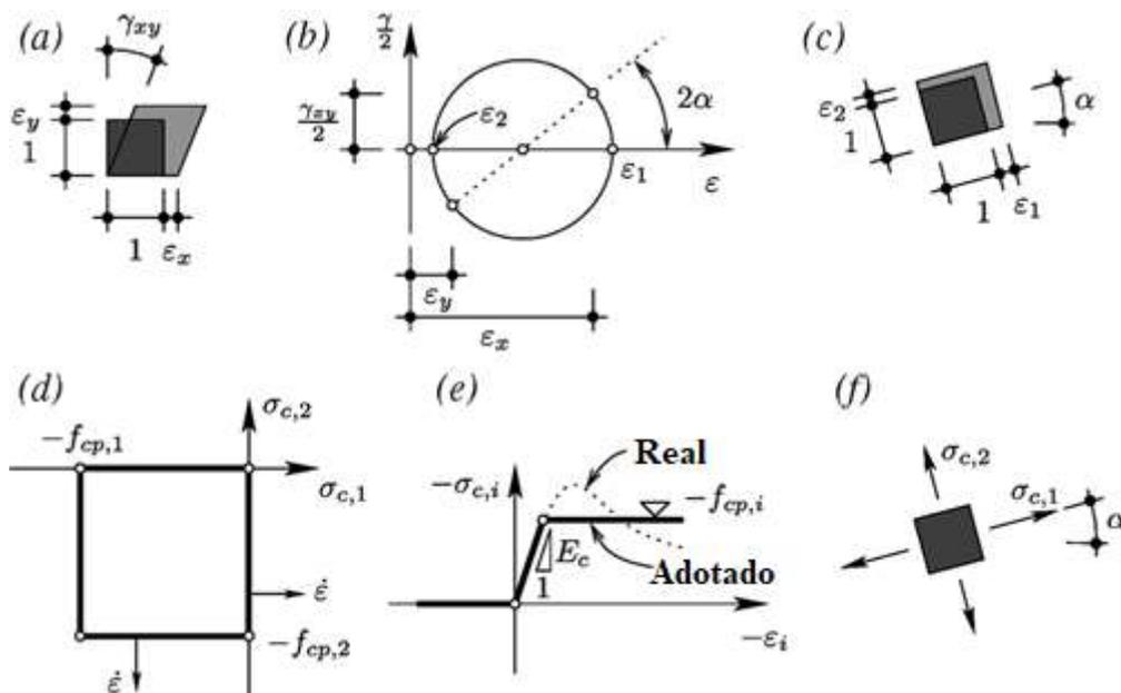
Figure 4 Principles for concrete modeling:
