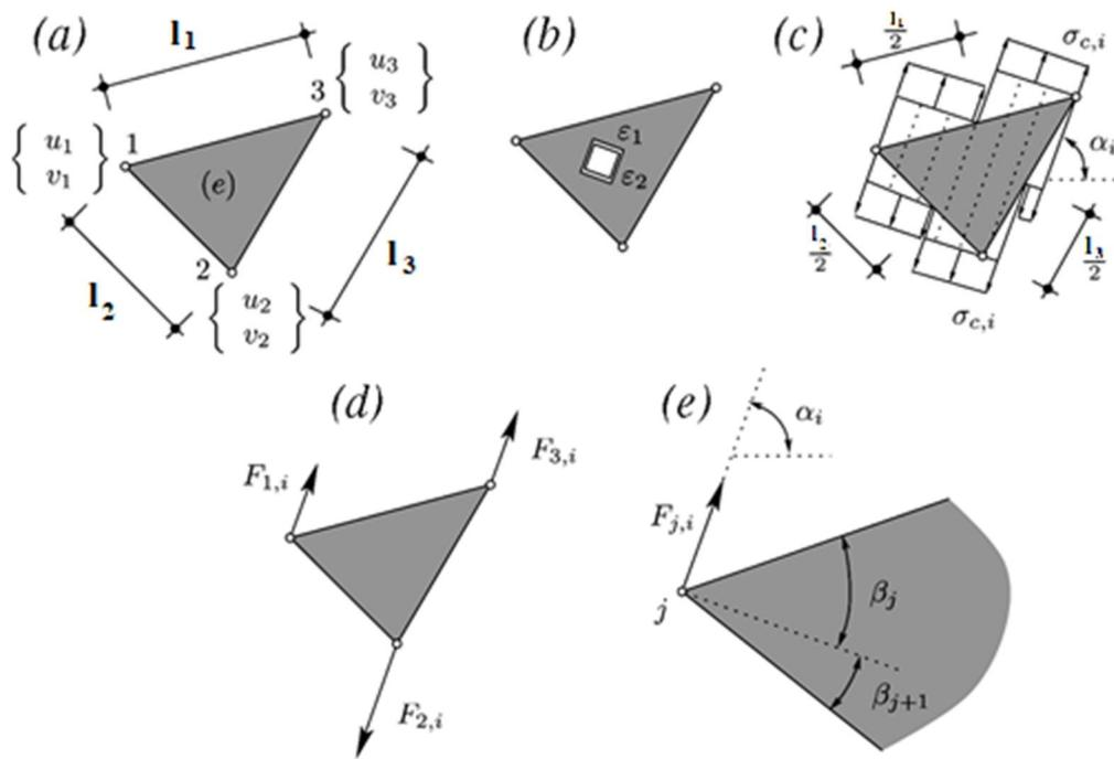
Figure 5 CST ('Constant Strain Triangle') Element
