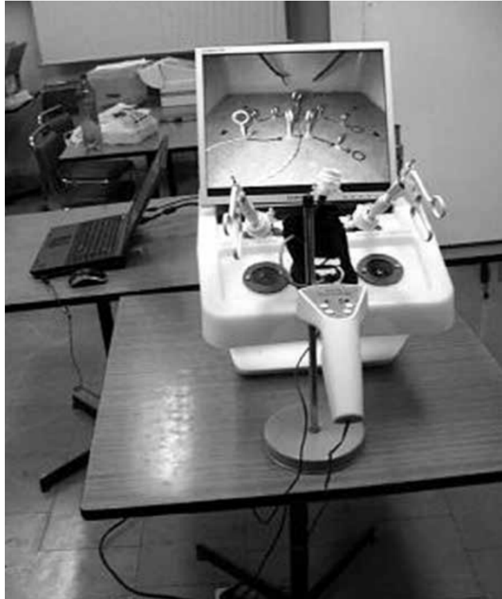
Figure 2.6: Walczak et al.'s second condition in their experimental setup had the screen positioned 20^\circ below eye level, 60cm away from the participant.
