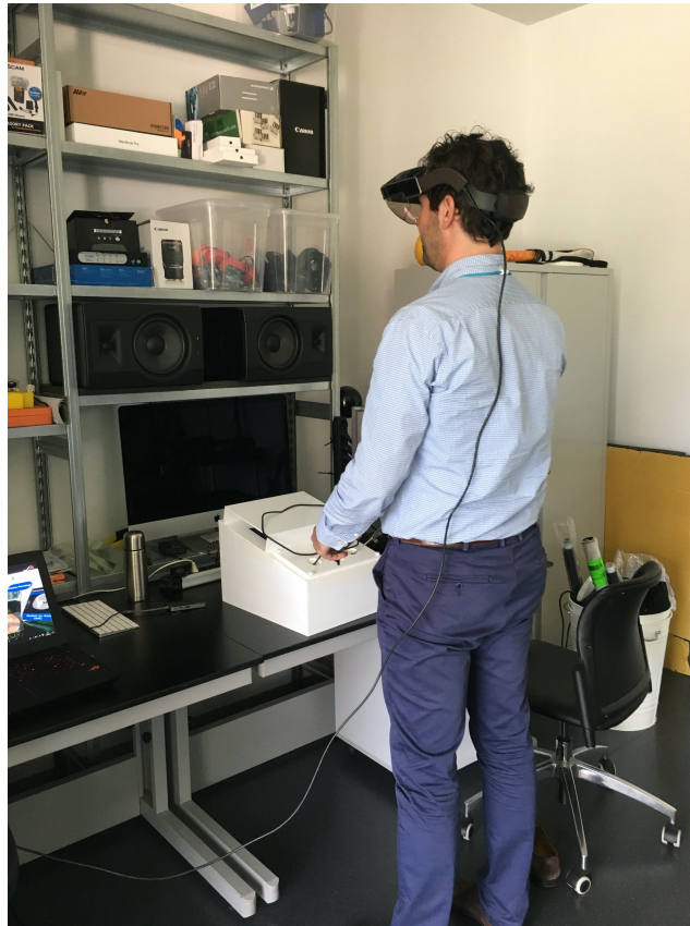
Figure 6.1: User in the exploration phase of the evaluation. Each hand holds a tool to confer a greater sense of authenticity and to prevent the user from rotating the torso as easily.
