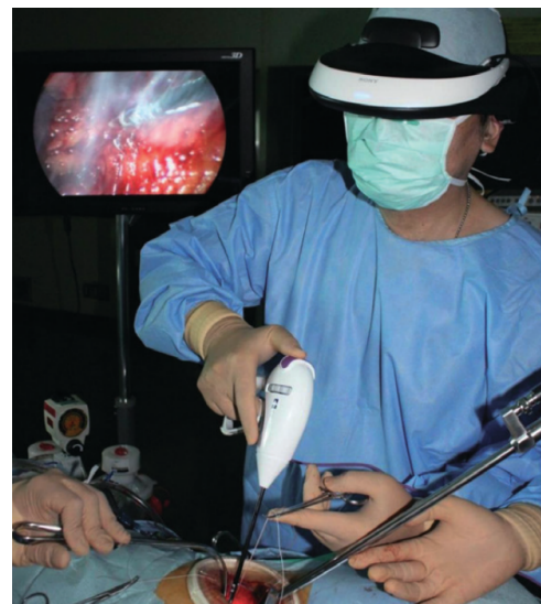
Figure 4: The HMD in Kihara et al.'s work allows visualisation of the hands and tools by looking down with the eyes.
