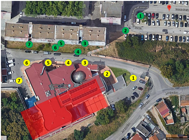
Fig. 14: Google geolocation API test in LATI. Yellow points real position; Green points Google estimated position; Red area represents area without Wi-Fi coverage.
