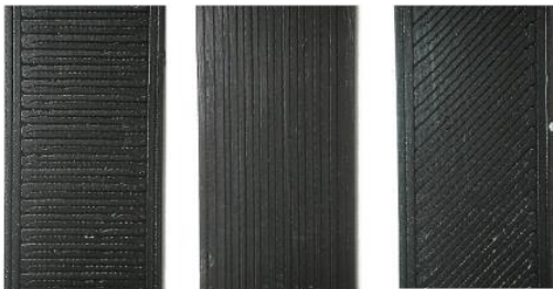
Figure 1: Deposition angle: 90° (left), 0° (middle) and 45° (right) [6]
