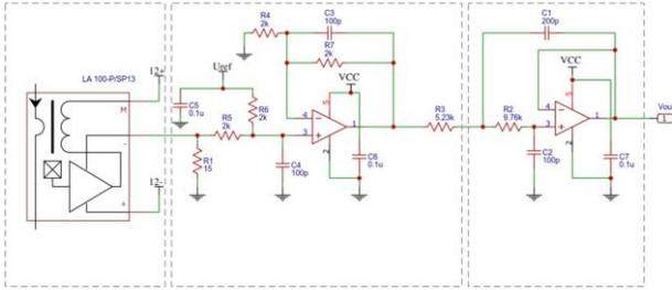
Figure 8 - Current Acquisition Circuit
