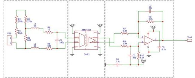
Figure 7 - Voltage Acquisition Circuit
