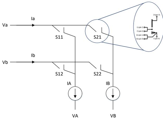
Figure 1 - Single-Phase Matrix Converter
