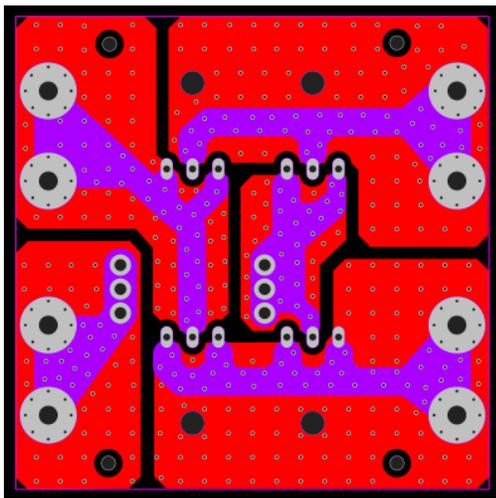
Figure 9- Full Bridge Rectifier layout
