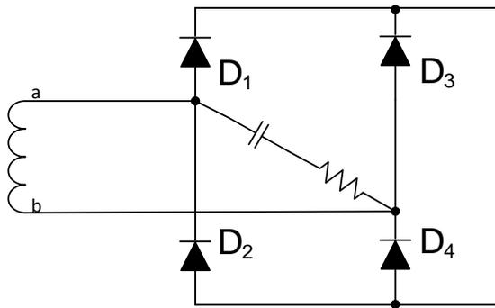
Figure 5 – Illustration of mounting of the snubbers on each rectifier bridge.
