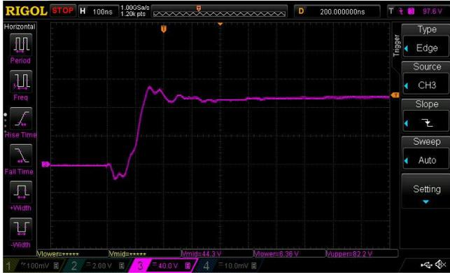
Figure 11 – Voltage  $v_{Ak}$  to diode terminals with snubbers
