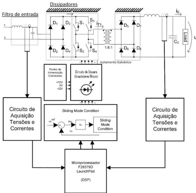
Figure 3– Matrix converter global schematic
