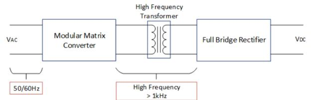
Figure 2 – Simplified scheme oh high frequency transformer
