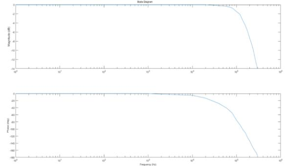
Figure 12 - Bode diagram of the current acquisition circuit
