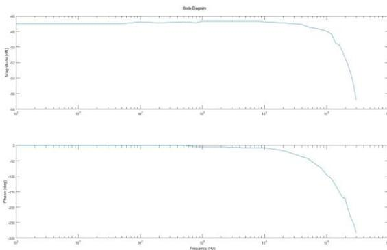
Figure 12 - Bode diagram of the voltage acquisition circuit
