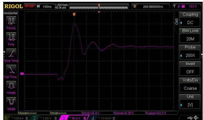
Figure 10 – Voltage  $v_{AK}$  to diode terminals without snubbers
