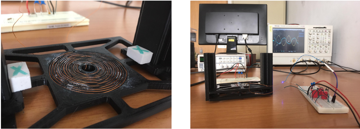
Figure 3.26: Left: 3D printed coil holding structure. Right: Experimental set-up.
