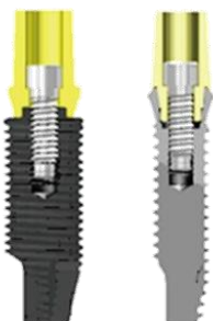
Figure 3.12. Cross sectional view of external ( left ) and internal ( right ) implants. Adapted from [56]
