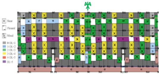
Figure 5 - Damage map of the back load-bearing façade wall P1 for the ultimate displacement along  $U_x$  direction.
