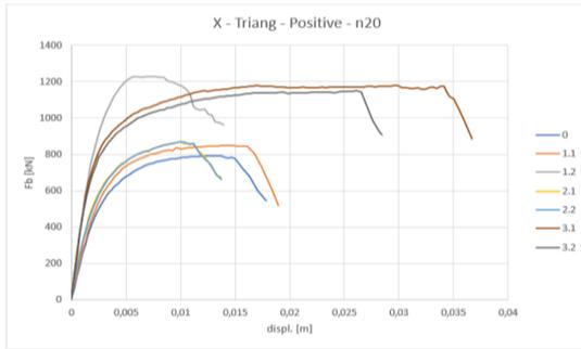
Figure 7 – Pushover curves from before retrofitting to solution 3.2, for the most demanding directions and corresponded load pattern.
