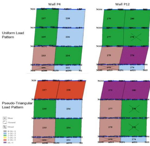
Figure 6 - Damage maps of the side wall P4 and shared wall P12 for the ultimate displacement along  $U_y$  direction.
