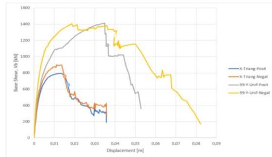
Figure 4 - Pushover curves for the case study building at its original state for both directions and considering the conditional cases of load pattern (dot mark the ultimate displacement considered).
