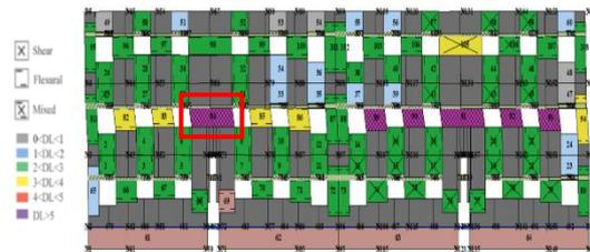
Figure 8 – Damage map of the back load-bearing façade wall P1 for the ultimate displacement along  $U_x$  direction.
