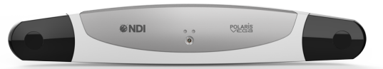
Figure 5: Polaris device used in the set up to perform the needed spatial calibrations.
