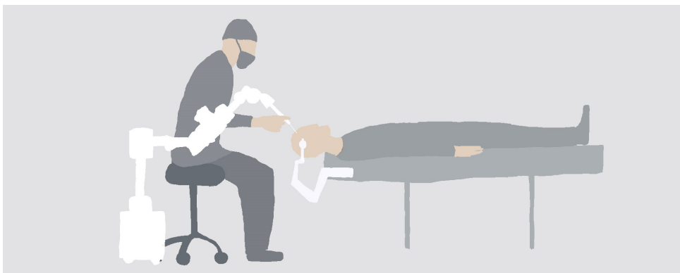
Figure 2.4: Shared control systems The surgeon controls the surgical tool but the robot uses its impedance interface so that the forces exerted between the surgeon and the end effector can be modeled as a second order system (adapted from Nathoo et al. [10])
