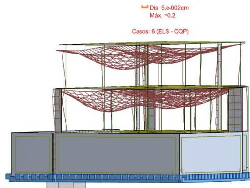
Figure 13 - Deformation in SLS
