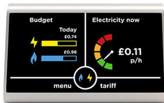
Figure 5.7 Smart meter, adapted from [41]
