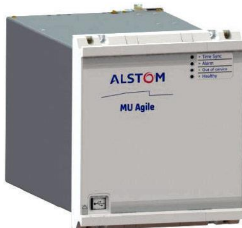
Figure 5.2 Merging unit, adapted from [35]
