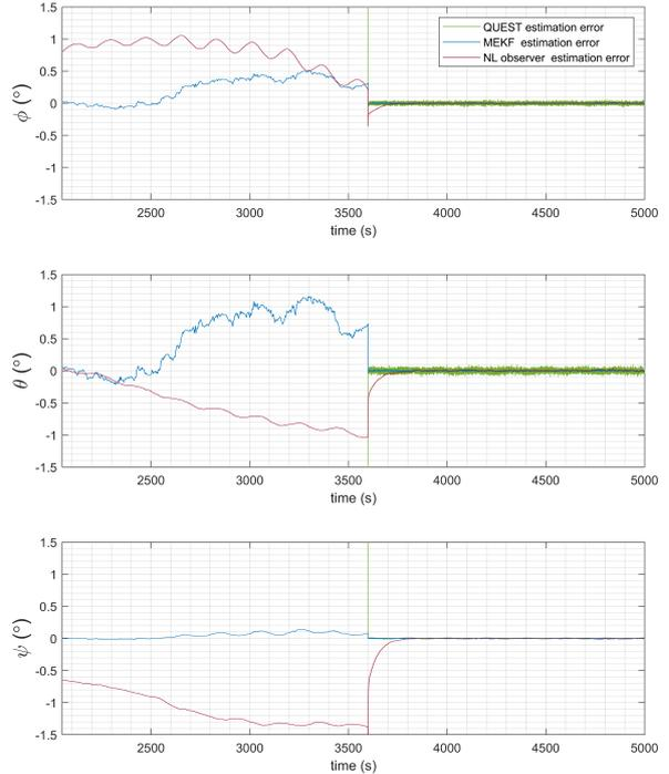
Figure 5: Detailed evolution of the angular estimation error for simulation case 4 with sensors reacquisition at 3600s.
