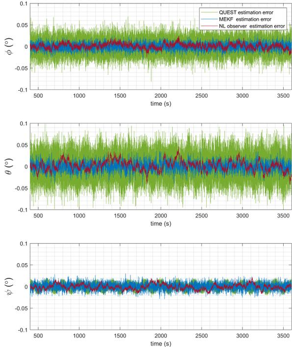
Figure 1: Detailed evolution of the angular estimation error for simulation case 1, orbit 1.
