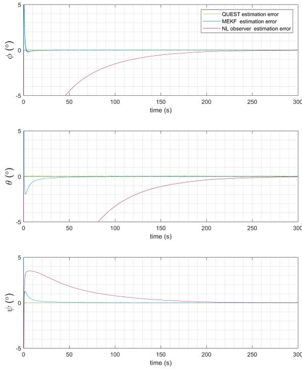
Figure 2: Initial convergence of the angular estimation error for simulation case 1, orbit 1.
