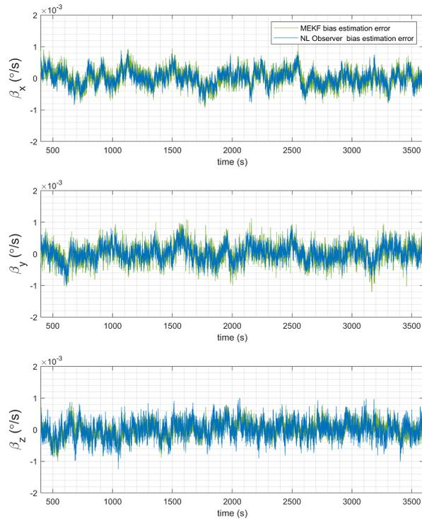
Figure 3: Detailed evolution of the bias estimation error for simulation case 1, orbit 1
