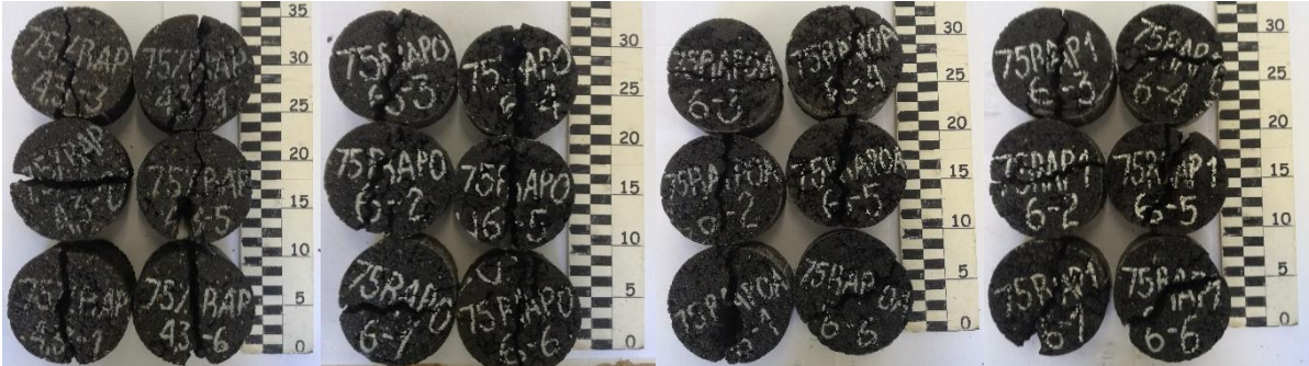
Figure 4.11: Cylindrical specimens used for the water sensitivity (from left to right: 75% RAP - M, 75% RAP, 75% RAP (Aged) and 75% RAP (2 nd phase))
