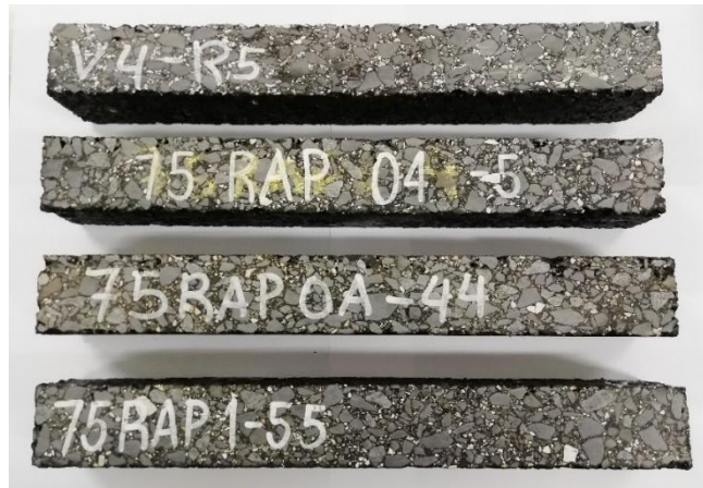
Figure 4.1: Beams in which were carried out the stiffness and fatigue resistance tests (from upper to lower: 0% RAP, 75% RAP, 75% RAP (Aged) and 75% RAP (2 nd phase))
