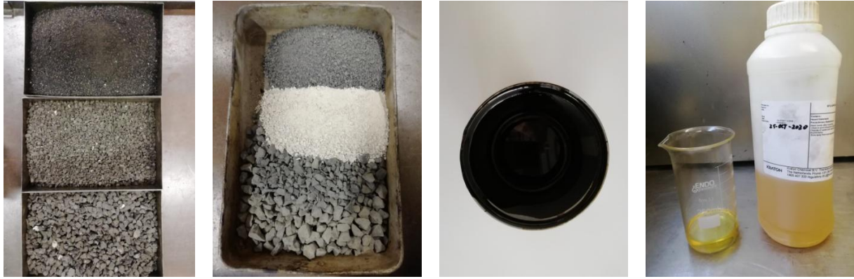
Figure 3.1: Components used to produce the recycled mixture (from left to right: RAP fractions, virgin aggregates, virgin bitumen and rejuvenator)
