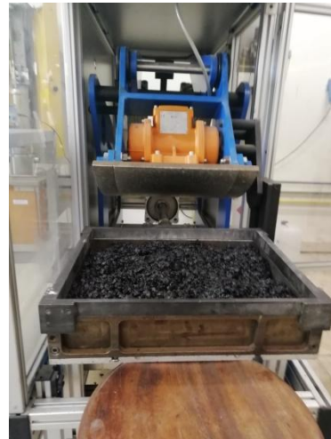
Figure 3.12: Steel roller compactor, with a loose bituminous mixture
