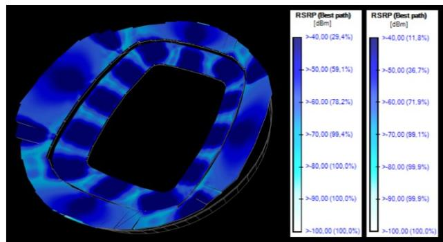
Figure 10 - Final solution iBwave RSRP output map obtained using the 2600 band.
