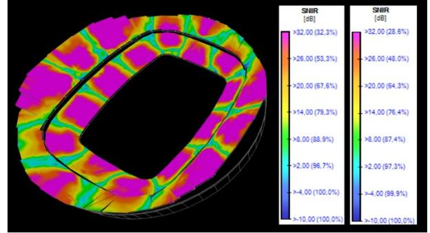
Figure 8 - Final solution iBwave SINR output map considering the 1800 MHz band.
