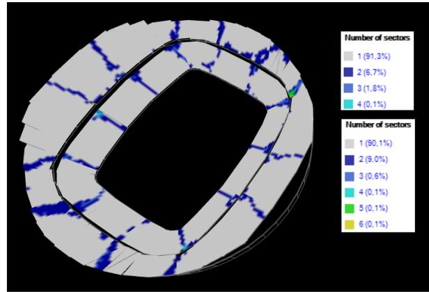
Figure 5 - Final simulation iBwave LTE Overlapping output map considering the 1800 MHz band.
