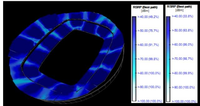
Figure 9 - Final Solution iBwave RSRP output map obtained using the 1800 band.
