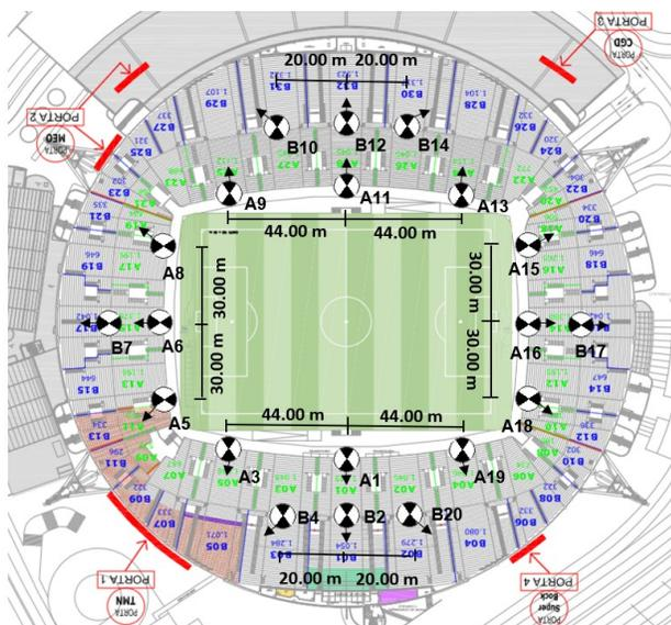
Figure 6 - Antenna final position scheme.
