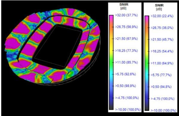
Figure 3 - iBwave SINR output map considering the 1800 MHz band (simulation 1).
