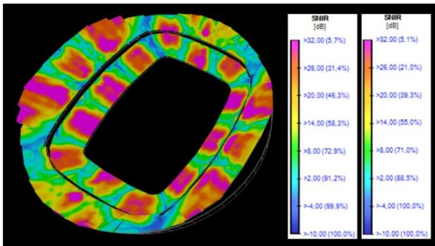
Figure 11 - Final solution iBwave SINR output map considering the 2600 MHz band.
