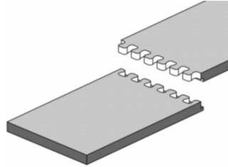
Figure 4 | Double lapped dovetail
