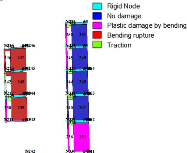
Figure 19 - Damage distribution for the severe damage displacement in the x direction, with the negative direction in an interior wall where structural changes occurred.
