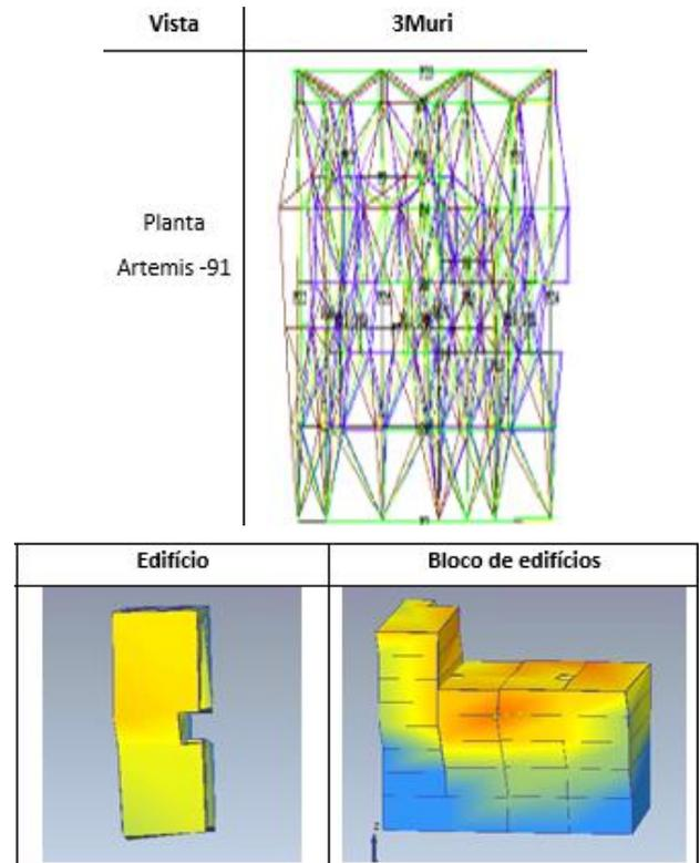
Figure 12 - Example of the comparison between the deformed shapes of the two models for a 2<sup>nd</sup> mode in x.
