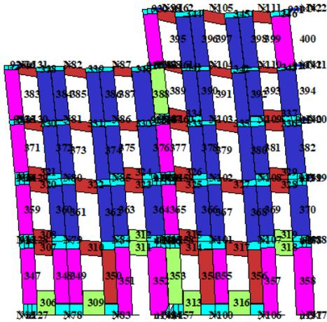
Figure 18 - Damage distribution for the severe damage displacement in the x direction, with the negative direction in the main façade.
