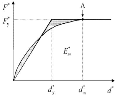
Figure 15 - Basic scheme of the bilinear curve.
