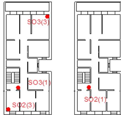
Figure 7 - Scheme with the locations of the free seismographs on the 1st and 2nd floors.
