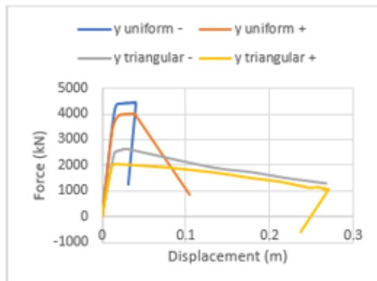
Figure 14 – Push-over curves for the negative direction.
