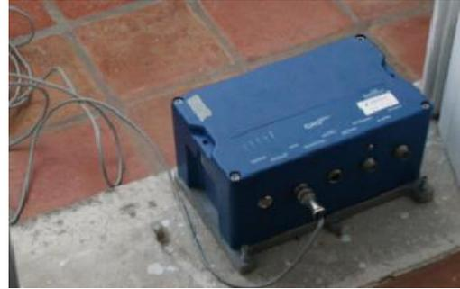
Figure 5 - Seismograph used in the tests.
