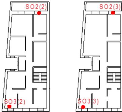
Figure 6 - Scheme with the locations of the free seismographs on the 2nd and 3rd floors.
