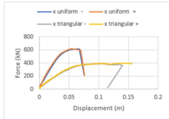
Figure 13 - Push-over curves for the positive direction
