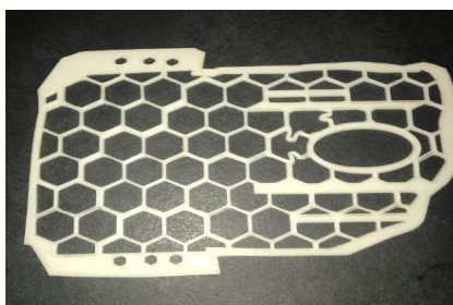
Figure 49 – 3D Printed arm cast with recycled PLA
