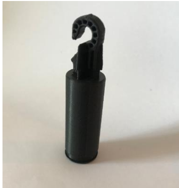
Figure 54 – 3D printed waterlock with recycled ABS
