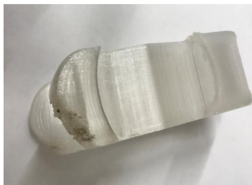
Figure 52 – Imperfections verified on the support
