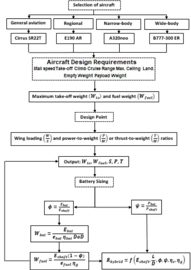
Figure 4: Hybrid-electric aircraft design procedure
