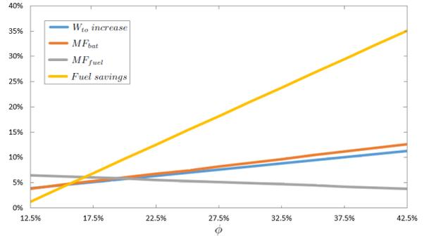
Figure 6: HEA-SR22T design operating with a 1200 W.h/kg Li-S battery with  $\phi$  variation
