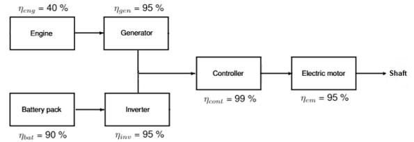
Figure 3: Hybrid-electric parallel configuration
