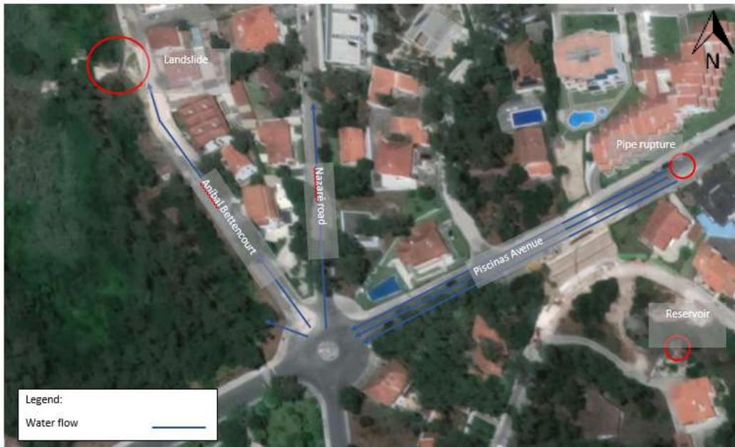
**FIGURE 1- WATER FLOW WITH LOCATION OF LANDSLIDE, WATER RESERVOIR AND RUPTURED PIPELINE (FERREIRA, ET AL., 2018)**
